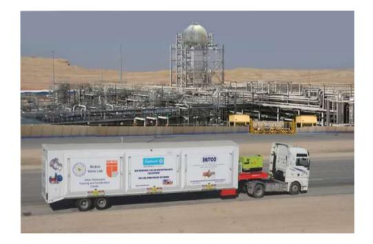
The mobile workshop facility includes Valve models including well head, ball, gate and plug valve of various size, Pressurized flow line, High pressure injection pumps and maintenance tools.
