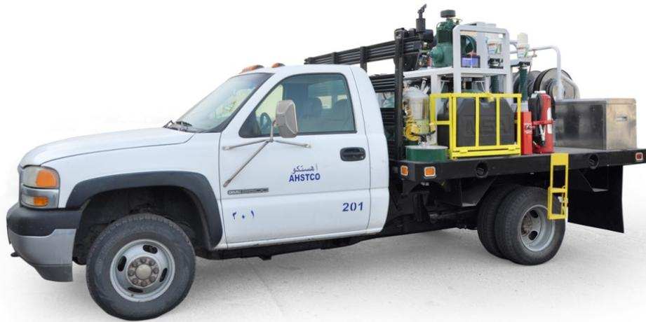
Sealweld can design and manufacture customized large volume and multiple unit pumps and air compressor packages for service trucks, valve service skids and offshore containers.
